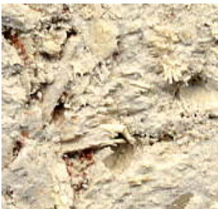
Figure 19: Matrix of 5:1 lime/hurd mix
