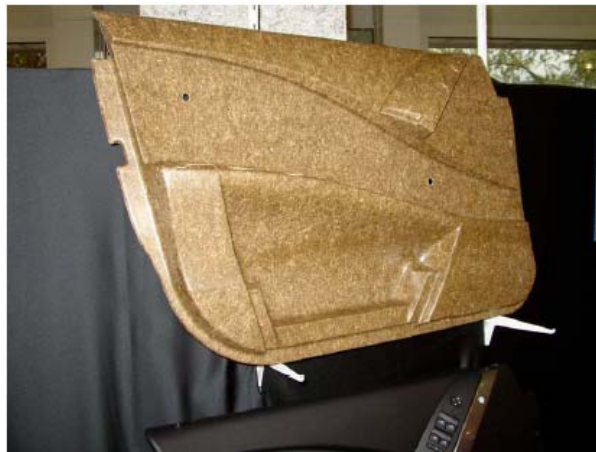
Figure 7: Example of inner car door made using hemp fibres (Nova Research Institute 2003)
